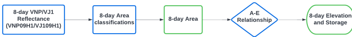
Figure 2. Flow chart of the algorithm for deriving the VNP28C2/VJ128C2 product, which contains 8-day area, elevation, and storage results for the 164 reservoirs. The product components are shown in green boxes.
